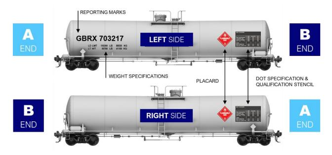
**CAR ENDS**. Tank car ends are designated "A" / "B", with the hand brake located on the Bend.
